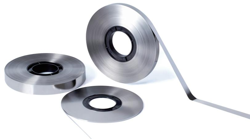
Fe-based Nanocrystalline alloys are based on Fe with Si and B with further additions of Nb and Cu. A subsequent heat treatment at crystallization temperature degree transforms the initially amorphous microstructure of the tape into the desired nanocrystalline state, this being fine crystalline grains (grains diameter of 10 - 20 nm only).
